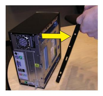
Release the two latching tabs on the left side of the front bezel by pulling them slightly outward. When the left side of the front bezel is released, pull it away from the computer.
